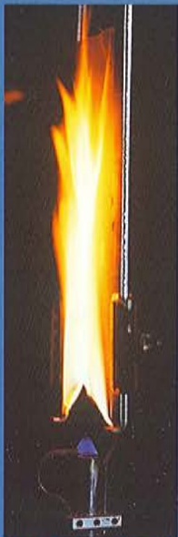
Vertical flame test on non-flame resistant fabric.
